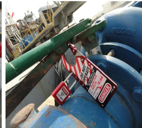
Pic 2: shows the safe practice to carry out Lock / Tag out in line with GDI procedure HSEMS.01/03.
