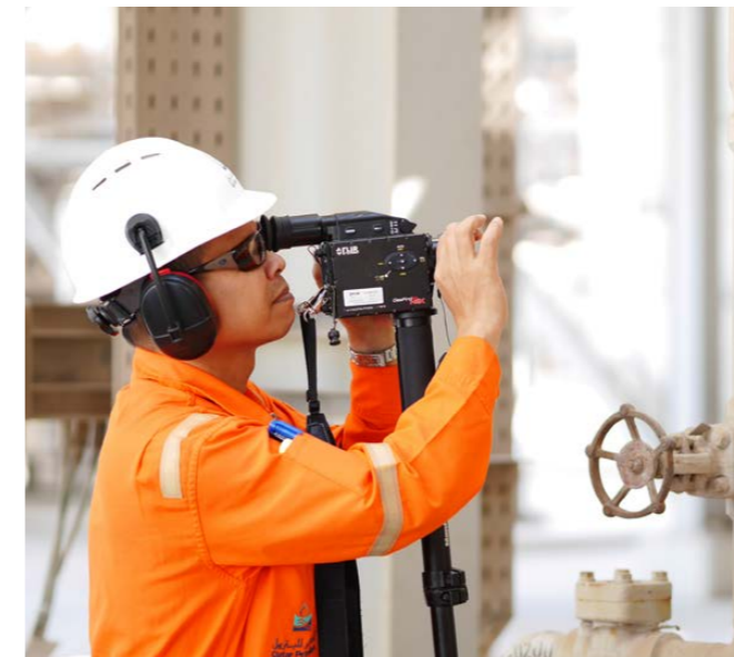
QP Operator using Infrared cameras for detection of fugitive Methane emissions
